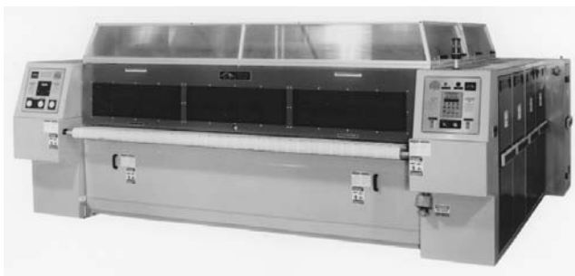
FIGURE 15.33 The Century Deep Chest All Roll Drive Flatwork Ironer is microprocessor controlled. (Photo courtesy of Chicago Dryer Company.)
