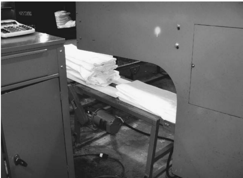
FIGURE 15.9 The towel is dispensed and automatically stacked on the other side. (Photograph courtesy of Mission Industries, Las Vegas.)
