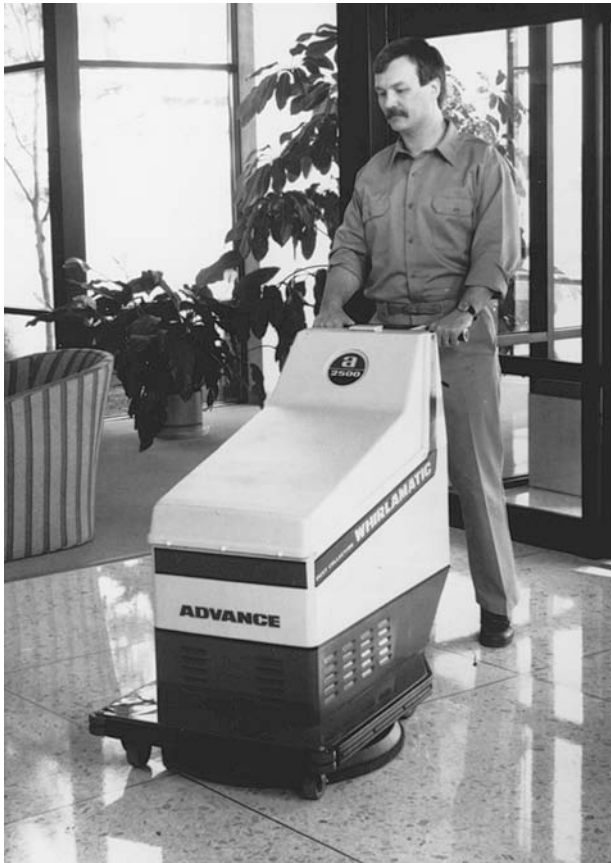
FIGURE 5.10 Burnishing a terrazzo floor. (Used with permission of the Advance Machine Company.)
