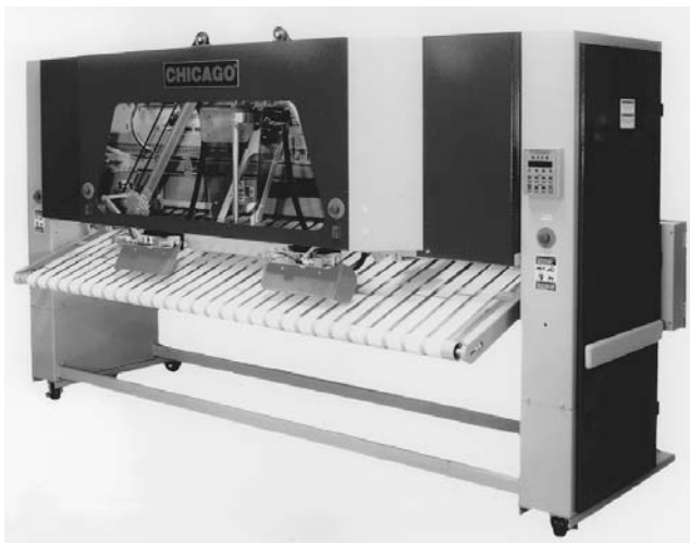
FIGURE 15.32 The King Edge accommodates not only sheets, but also other flatwork items such as pillowcases, napkins, and tablecloths on the bypass conveyor. (Photo courtesy of Chicago Dryer Company.)
