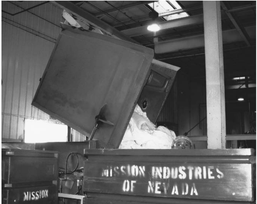
FIGURE 15.2 A mechanical arm lifts a laundry cart, dumping its contents onto a conveyor belt. An average of 1200 of these carts arrive at this plant every day. (Photograph courtesy of Mission Industries, Las Vegas.)
