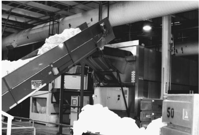
FIGURE 15.4 The sorted laundry goes up a conveyor into a tunnel washer. These machines can wash up to 3,400 pounds of soiled laundry per hour. There are seven of these tunnel washers at this plant. (Photograph courtesy of Mission Industries, Las Vegas.)
