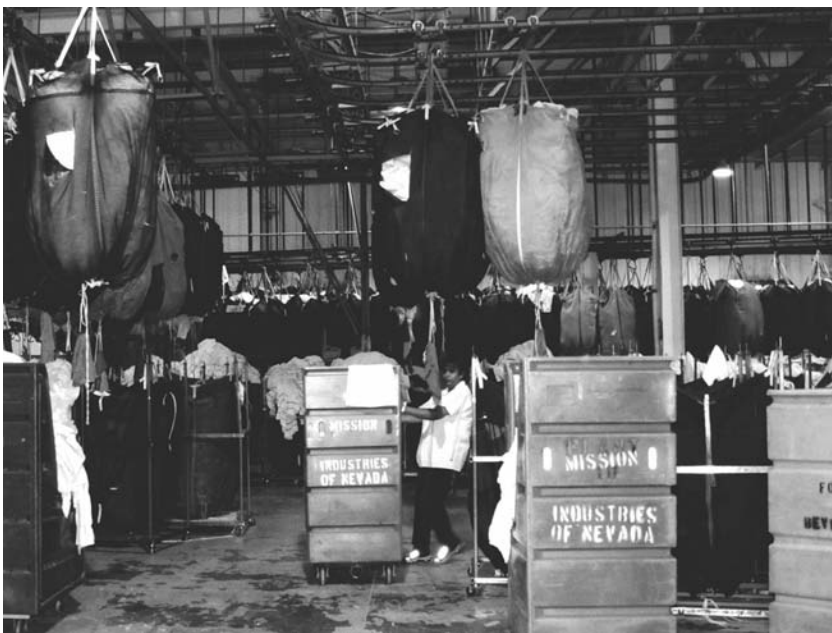
FIGURE 15.15 Some of the linen is not shot through tubes, but moved in giant laundry bags on an overhead conveyor system. The linen is emptied by releasing a drawstring on the bottom. (Photograph courtesy of Mission Industries, Las Vegas.)
