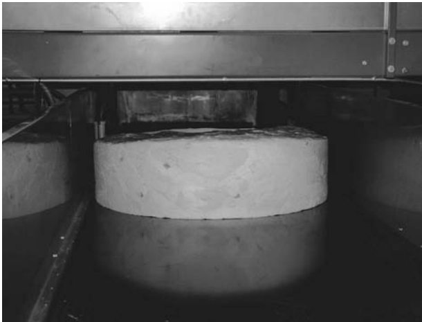
FIGURE 15.5 After washing, the laundry is pressed to extract water from the fabric. The washer dispenses the clean laundry in the form of 110-pound cakes. The largest tunnel washer produces a 220-pound cake. (Photograph courtesy of Mission Industries, Las Vegas.)
