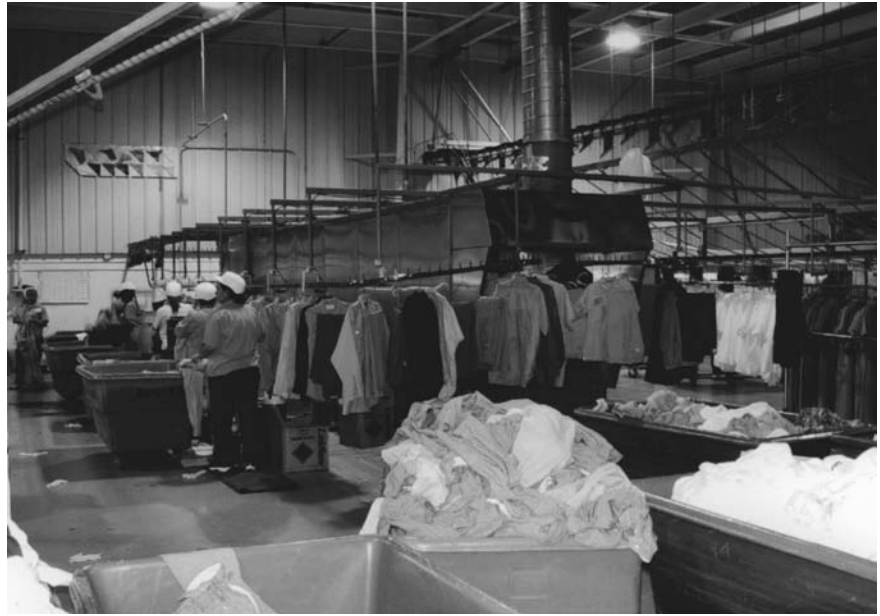
FIGURE 15.19 Laundered uniforms enter a large steamer; when they come out, the wrinkles are gone. (Photograph courtesy of Mission Industries, Las Vegas.)
