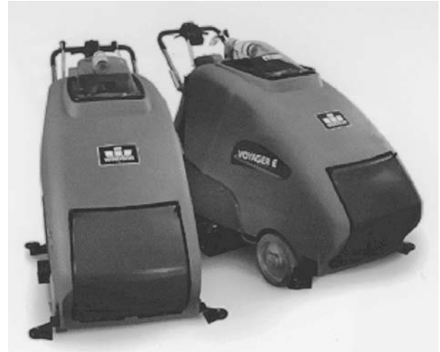
FIGURE 6.31 The Voyager E from Windsor® features a 40-gallon solution tank that can clean 8100 square feet of carpet per hour. (Photo courtesy of Windsor Industries, a Castle Rock Company, Englewood, Colorado.)
