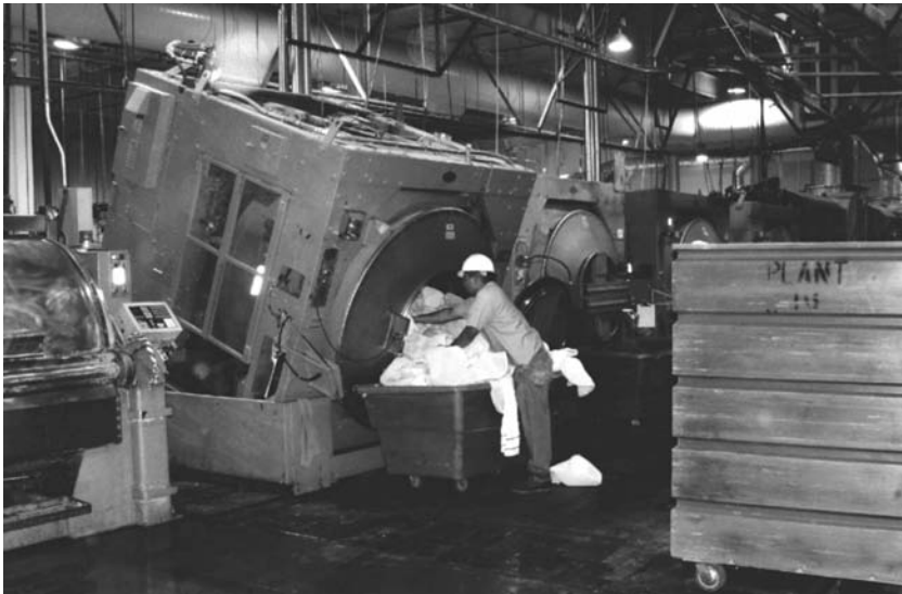
FIGURE 15.14 Here one of the mid-sized washers is being emptied. Note how the washer tips to aid the worker in emptying the machine. (Photograph courtesy of Mission Industries, Las Vegas.)
