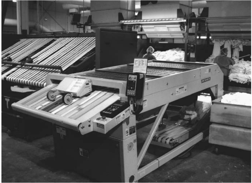
FIGURE 15.17 This state-of-the-art folder can fold all sizes of towels with just a push of a button. (Photograph courtesy of Mission Industries, Las Vegas.)
